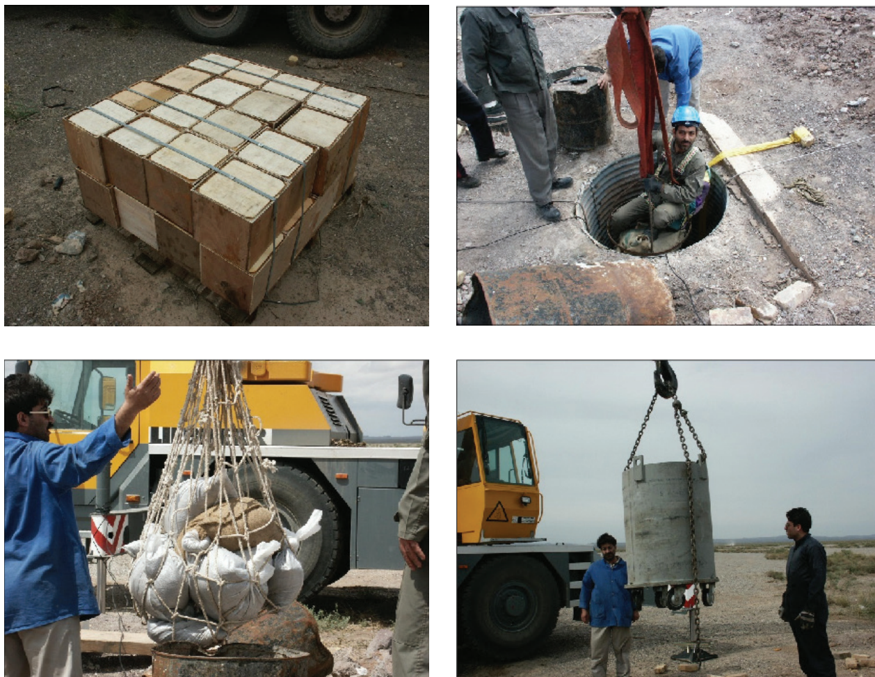
Figure 22. Archive images of high explosive tests. High explosives in upper left image. High explosive shaft (upper right). Possibly fill material for the shaft (bottom left) and capping it with a concrete plug, prior to detonation (bottom right).
